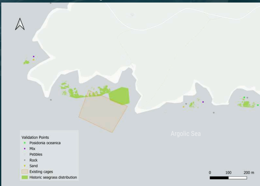
Figure 21. Aol 3 with the historic meadows shown in green, habitats indicated by coloured dots, and aquaculture cages visible.
